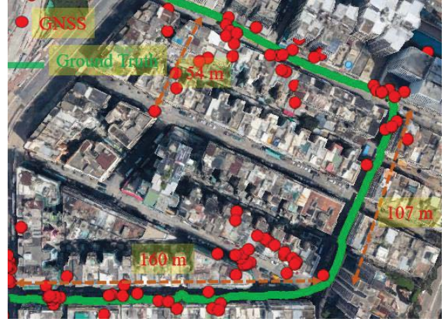
Fig. 9. The trajectory of the autonomous vehicle is indicated by the green curve. The red circles indicate the GNSS positioning result [32].
