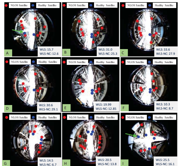
Fig. 12. Illustration of Skyplot which indicates the satellite distribution during the dynamic experiment. The green circle represents the satellites that are healthy. The red circle denotes the NLOS satellites [41].
